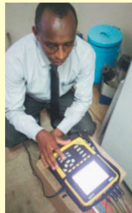
Peter Waturo of ERC takes a reading from a power analyzer during an energy audit carried out at Eagle Africa centre, the building that hosts the commission's offices.
